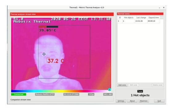
You will set the value Temperature calibration to Static Calibration and set the value of Temperature Static Deviation to minus 0.6 degrees.
