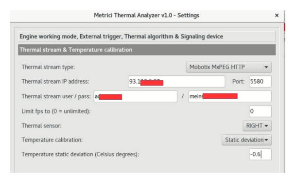
So Metrici will substract 0.6 degrees from every temperature offered by the thermal camera.
