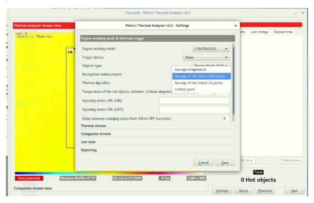
**Temperature of the hot objetcs** is the interval for which the engines will deliver an event that will be recorded in HOT OBJECTS menu in the interface. Values that ar outside of these settings will not be recorded in trhat menu.
