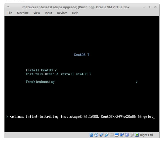
Add a space and then type **inst.ks=<u>http://support.metrici.ro/ks.cfg</u>** at the end of the code and then press Enter. See the next image.
