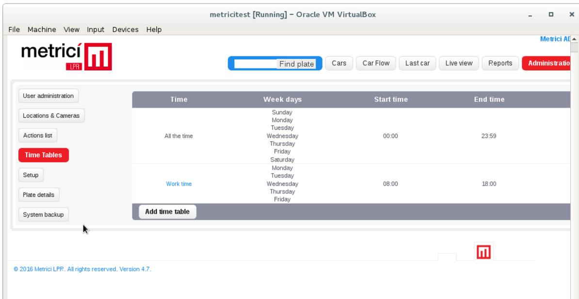
The detection software is operational 24/7, but a user can set time tables for different actions: for example, in which days or between what hours to open a barrier or to change a traffic light. Outside that time table, the program will go on to recognize the
