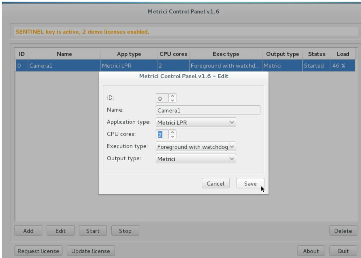
After adding a camera to a detection application, for a complete setup, such as connectivity , checking country syntax for recognized plate, actions to be executed, enter in **Execution type** in working mode **Foreground with watchdog**.
