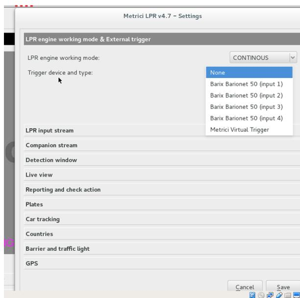
Keep in mind that when setting the detection with trigger you can also choose how many seconds the LPR engines is trying to detect a number plate. See next image. In case there is no number plate or this is not visible, dirty, partial etc., Metrici LPR engine will generate an event and will be added to database with the ID UNKNOWN. This will be accompanied by a still frame that you can check and see if there was a vehicle or not.
