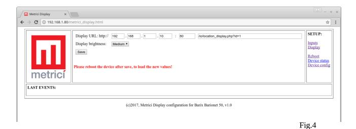
In the **Display** option URL you will fill the IP address of Metrici server, the port of connection, followed by the string generated by the application such as /io/location\_display.php?id=1. Where "id=" is the a number of a location, that is automatically generated by the software. This is to be consulted in Administration-Locations&Cameras-NAME OF THE LOCATION-Edit parameters.
