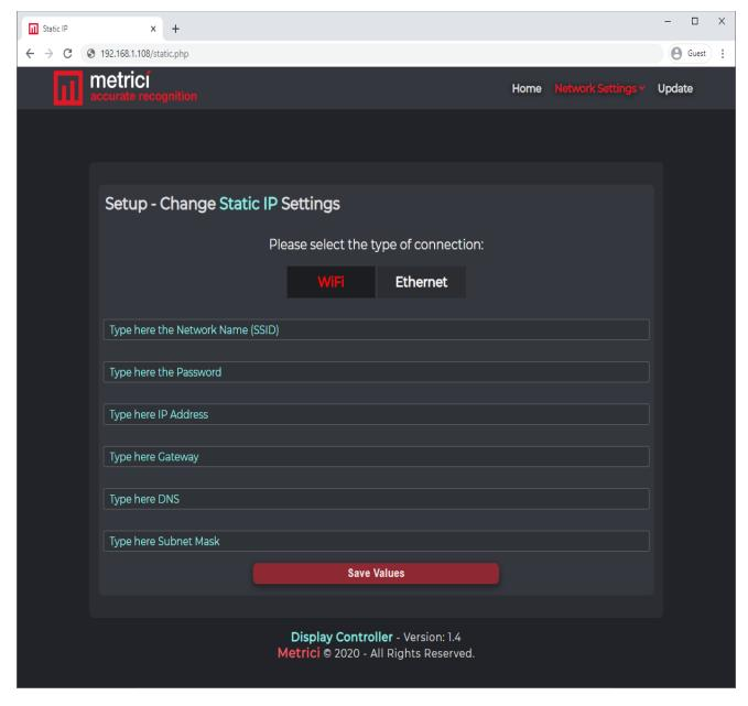
If you choose Ethernet, the fields you have to fill in are the IP ADDRESS, GATEWAY, DNS and SUBNET MASK.
